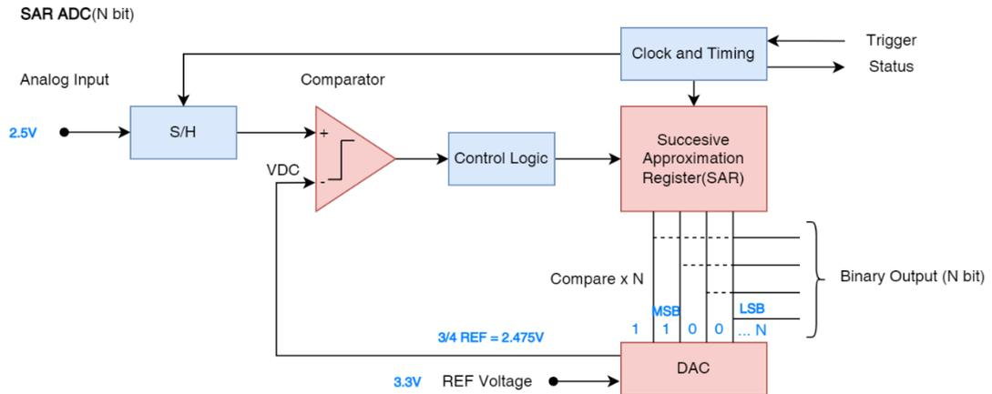
Figure 8 ADC Conversion Approximation Step 2
