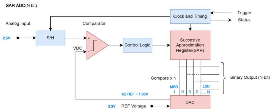
Figure 7 ADC Conversion Approximation Step 1
